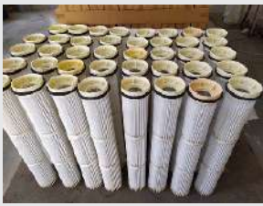
RMC Plant Silo Filter
